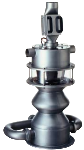
Cascade separator with integrated metal separator and ionizer. Thanks to the special design, fine dust and impurities adhering to the pellet surface are separated from the raw material. One of the basic elements for avoiding impurities in a reliable way.
