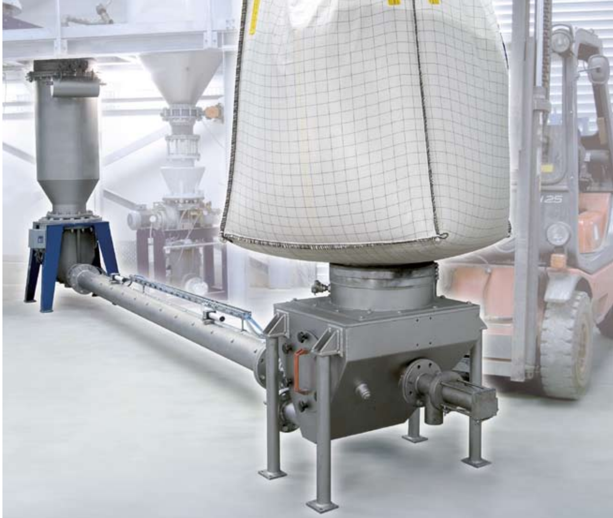
Demonstration plant in our Technology Center. Right: feeding of bulk solids from Big Bags. Left: Pump-Flow feeding station. Maximum conveying distance is 300 m, optionally dilute phase or dense phase conveying.
