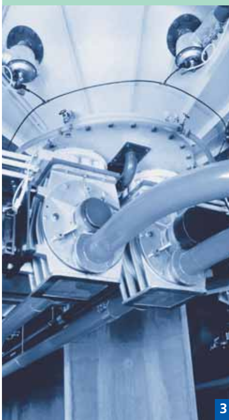
Picture 3: Parallel production lines from a single silo, enabled by a flat fluidizing bed design (up to 4 outlets possible)
