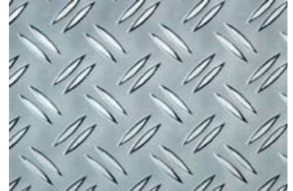
Thanks to the structured surface of the plate the wall friction coefficient is changed.
